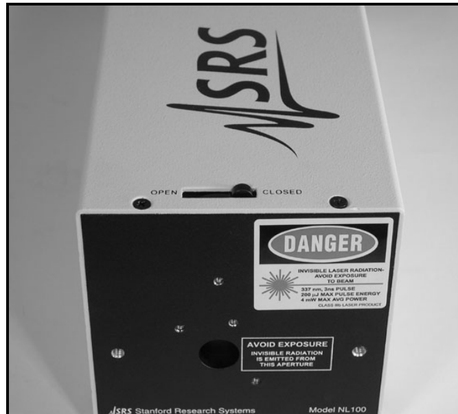
Figure 14. Front of the NL100 laser system, showing the beam shutter in the closed position.
