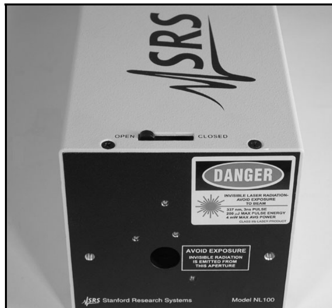
Figure 15. Front of the NL100 laser system, showing the beam shutter in the open position.
